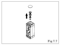
Remove the cushion, and then push out the spool assembly from opposite side. [Fig.7.7]
