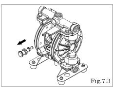
Remove Spool assembly by pushing it from Cap A side (the side without reset button). [Fig.7.3]
