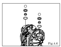
• Remove the Ball, valve seat A, valve seat B, O ring. [Fig.4.6]
