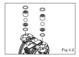
• Remove the O ring, valve stopper, ball, valve seat. [Fig.4.2]
