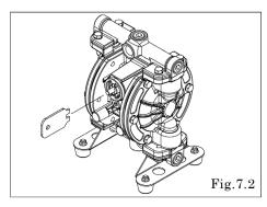
Remove the cap A and cap B using the cap remover. (special tool: Part No. 717114). [Fig.7.2]
