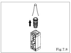
• Remove the sleeve using the sleeve remover (special tool: Part number 713148). [Fig.7.8]
