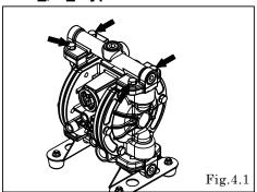
Remove 4 mounting bolts from upper manifold and remove the manifold. [Fig.4.1]
