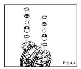
• Remove the O ring, valve seat, ball, valve stopper. [Fig.4.4]
