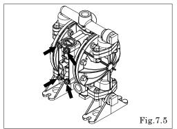
Remove 4 nuts fixing the valve body assembly and draw out the valve body assembly from the main body. [Fig.7.5]
