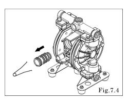
• Remove the sleeve using the sleeve remover (special tool: Part number 713148). [Fig.7.4]
