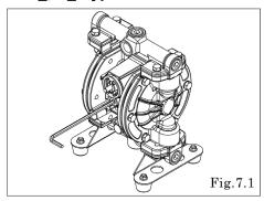
Loosen the plug with hexagonal box wrench and remove remaining air from inside the pump. [Fig.7.1]
