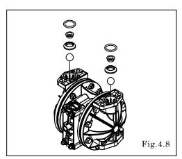
• Remove the O ring, valve seat B, valve seat A, ball. [Fig.4.8]
