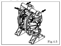
Remove 4 mounting bolts from upper manifold A and remove the manifold A. [Fig.4.5]
